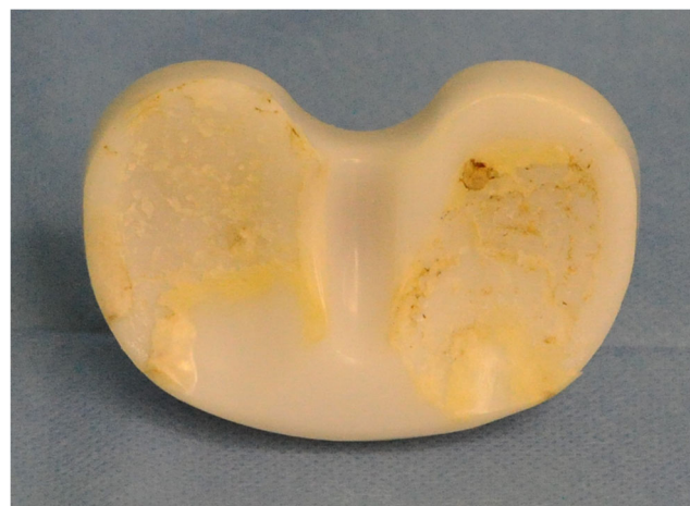
Fig. 2 Intra-operative picture of a polyethylene insert 148 months after implantation with medial and lateral delamination
